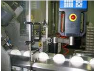
Cheese being wrapped by the automatic packaging machine
